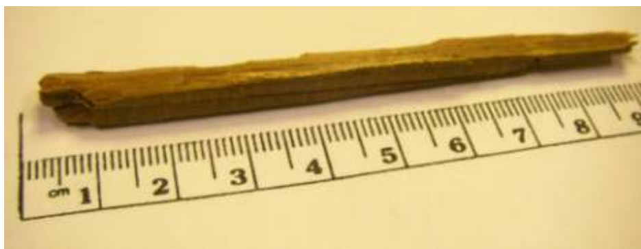
Figure 219. Large Cedar Woodchip with Splitwood Characteristics.
